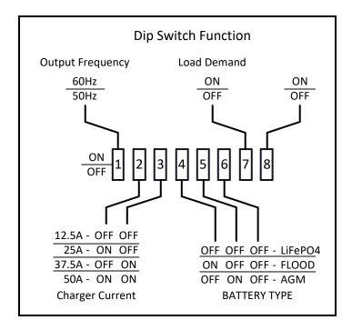
The factory DIP Switch settings are: 1, 2, 3, 4 and 8, ON (UP); 5, 6 and 7, OFF (DOWN).
