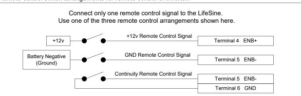
Note: The LifeSine is designed to accept ONLY ONE remote control signal. If more than one of the signals shown above are connected to the inverter, it won't harm the LifeStar but would provide undesirable operation since the signals will be performing "in parallel".
