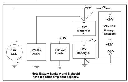
output. When a 12 volt load is present, and Battery A's voltage decreases to just below the voltage of Battery B, the battery equalizer activates and transfers sufficient current from Battery B to Battery A, satisfying the load and maintaining an equal voltage and charge in both batteries.
